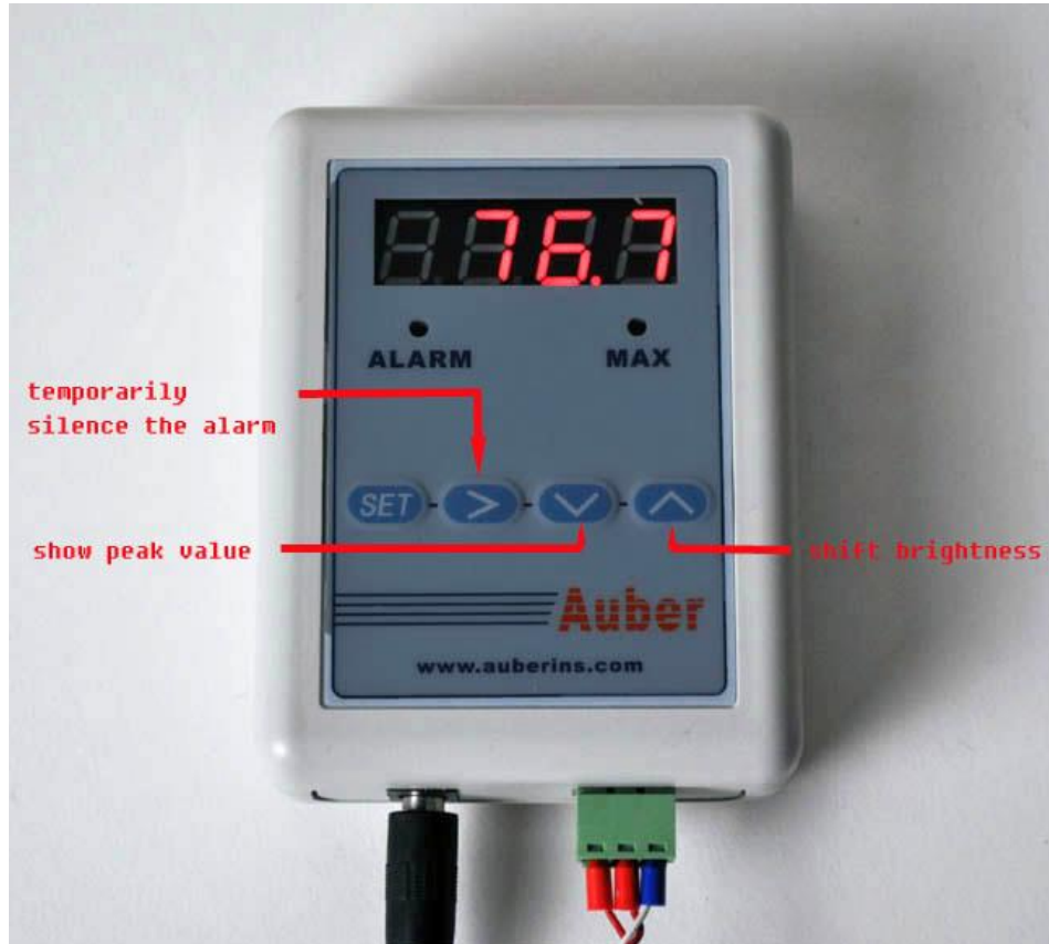
Figure 2 Function keys during temperature measurement operation
