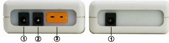
① Power Input - 12VDC power supply input (2.1 mm O.D.). ② Power Output - 12VDC output (2.5 mm O.D.). ③ Probe Input - temperature probe input
