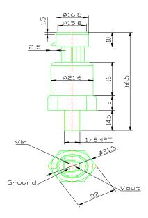
This pressure transmitter is to be powered by regulated 5 VDC power supply. Connect red wire to the 5VDC power source. Connect black wire to the ground. Green wire is the signal output.
