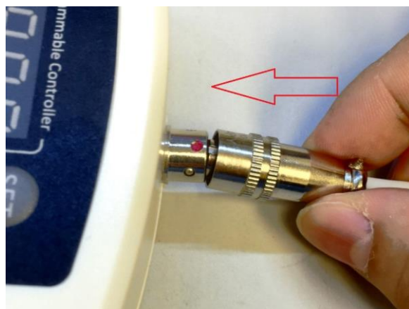
Figure 5. Install the sensor.
