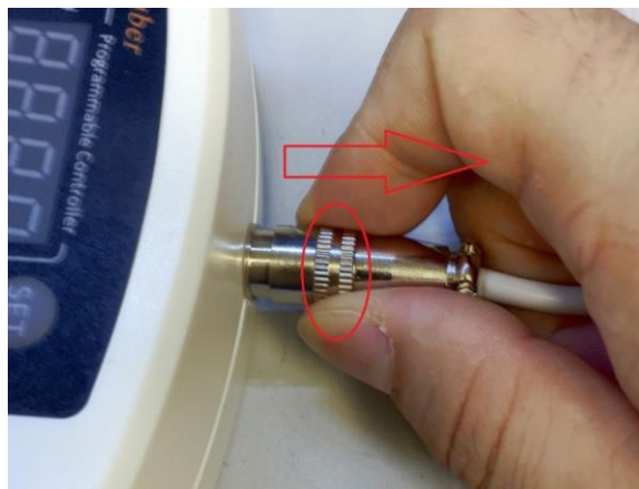
Figure 6. Remove the sensor.
