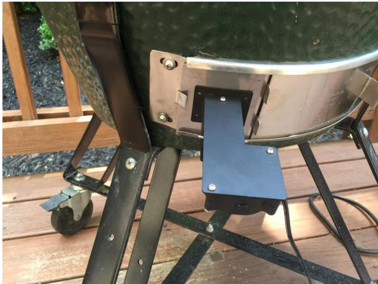
Figure 4. Mount the blower with the fan facing downwards.
