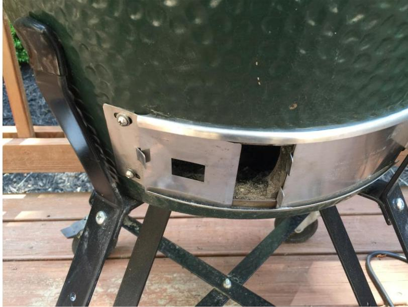
Figure 2. Insert the adapter plate to the lower vent.
