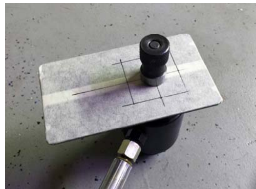
Figure 6. (b) Install the of the 22 mm die on the hydraulic knockout punch driver. (c) Assemble and panel, punch, and nut onto the draw stud.
