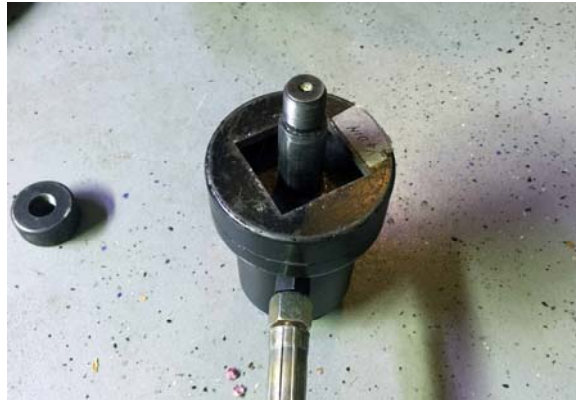
Figure 7(a). Install the 1/16 DIN die on the hydraulic knockout punch driver.
