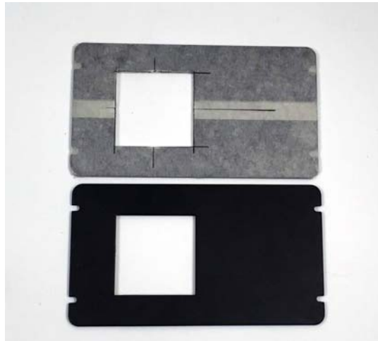
Figure 8. This is a picture of punched panel (top) compared with a factory pre-punched panel (bottom).
