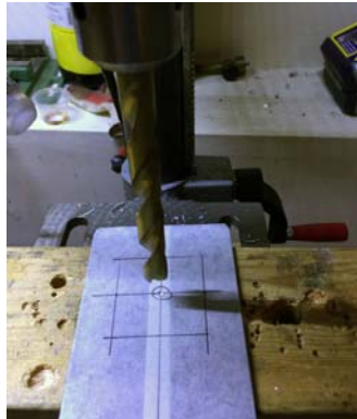
Figure 6(a). Drill a small pilot hole on a drill press with a 7/16" drill bit.
