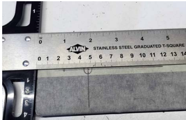
Figure 3. Find the center and draw two reference lines.
