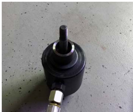
Figure 6. (b) Install the of the 22 mm die on the hydraulic knockout punch driver. (c) Assemble and panel, punch, and nut onto the draw stud.
