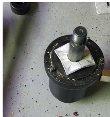
Figure 7. (b) Assemble the panel, punch, and the nut onto the draw stud. (c) Remove the top section of the die so that the knockout piece can be extracted.
