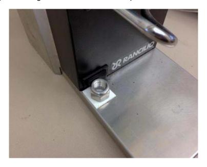
Figure 1, a simple way to hold the push and hold switch of Rocky at the on position. A screw nut is held in place by a double sided tape.
