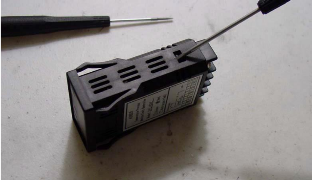
Fig 1. Gently insert a small screw drive. Don't press too hard. Otherwise the tap will break.
