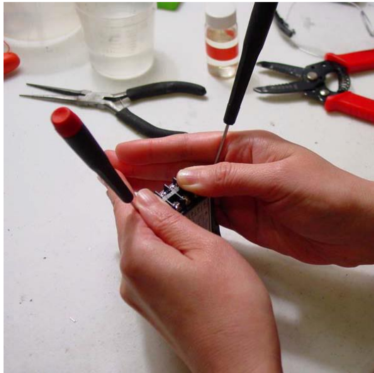
Fig 1. Gently insert a small screw drive. Don't press too hard. Otherwise the tap will break.
