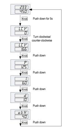
Figure 2. Flow chart of how to change the parameters under code 166. This is an example of RDK200/300 controller.
