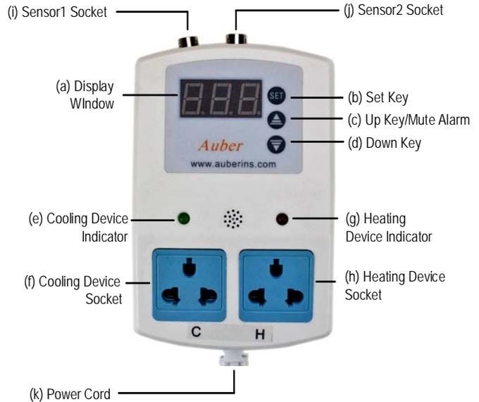
Figure 1. Front panel of TD300.
