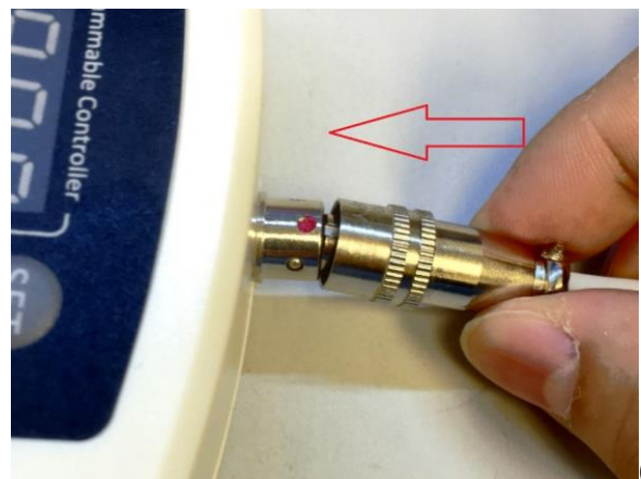
Figure 4. Install the sensor.
