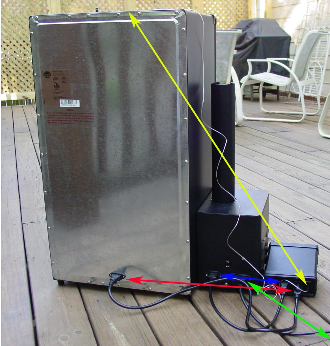
Fig 14. Power connection of the controller and smoker. The generator is connected to the power strip by the power cord from Bradley (green arrows). The input of the controller is connected to the female receptacle on the generator by the power jumper cord provided by the Bradley (blue arrows). It is the cord that used to connect the generator to smoker. The controller output is connected to the smoker by the power cord (red arrows).
