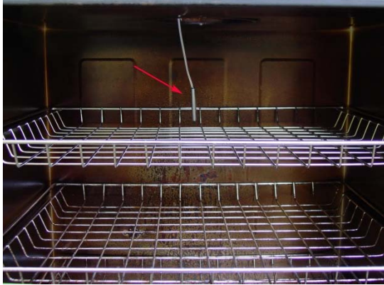
Fig 15. Sensor position. Left, the sensor should be placed close to the food but high enough so that it does not touch the food. Right, hold the sensor in place with a piece of tape.
