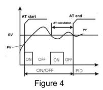
Before using the auto-tune function, you must set the cooking equipment up in the exact configuration it will be used. For example, to tune a rice cooker, place the sensor in the room temperature pot filled with water and plug the cooker into the
