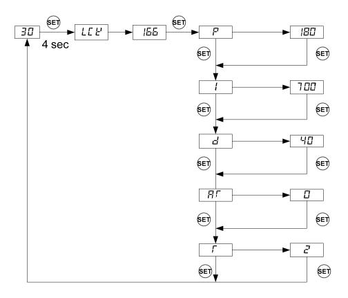
Figure 4. Code 166 Parameter setup flow chart
