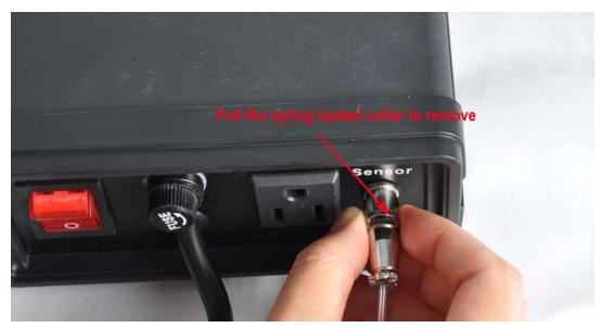
Fig 3b. How to remove the sensor.
