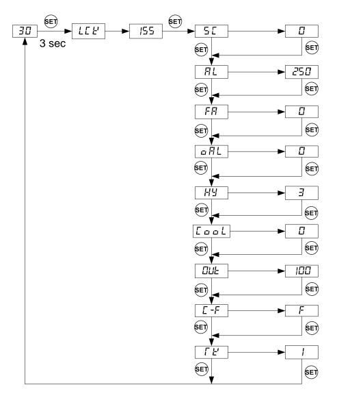
Figure 5. Code 155 Parameter setup flow chart
