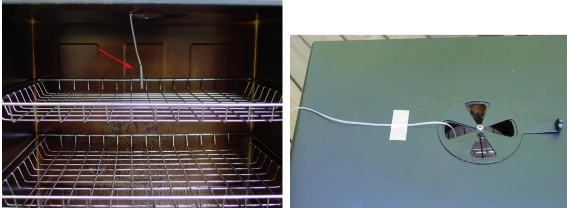
Figure 5. Sensor position. Left, the sensor should be placed close to the food but high enough so that it does not touch the food. Right, hold the sensor in place by a piece of tape.
